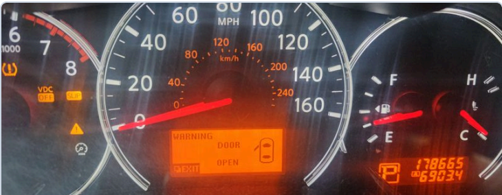
Plate 2: Instrument Cluster Telemetry 178,665 verified miles. VDC OFF and SLIP indicators illuminated under ECM torque failsafe.
