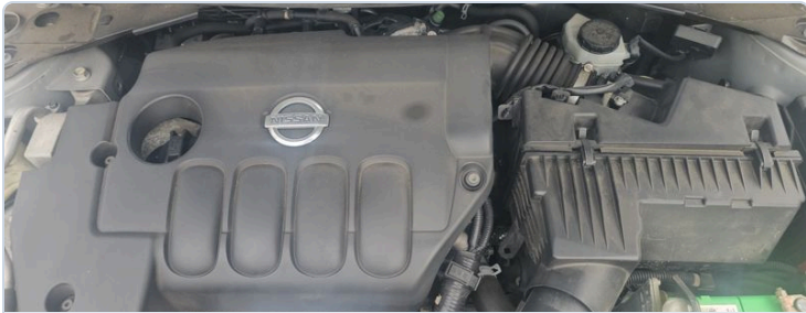
Plate 3: QR25DE 2.5L Engine Bay Layout Cylinders 1-4 left-to-right. Cylinder #3 is located under the 3rd contour runner of the engine cover.
