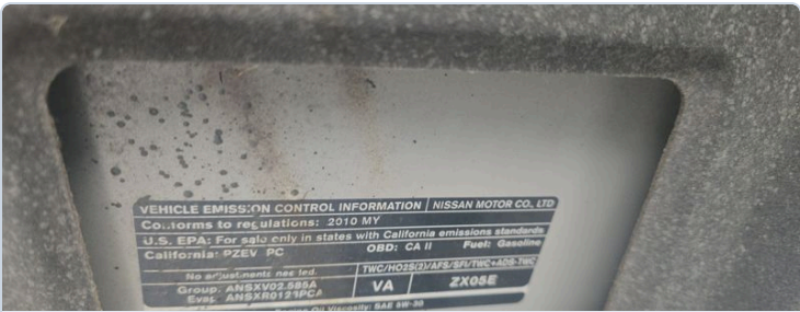
Plate 6: Underhood Emissions Certification 2010 MY Nissan California PZEV PC certification (Group: ANSXV02.585A, SAE 5W-30 oil specification).
