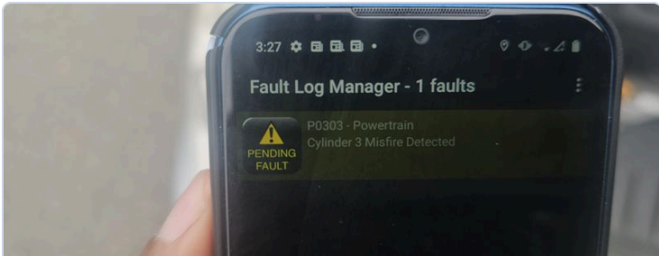
Plate 1: OBD2 Scan - Torque Pro Fault Log Confirmed active P0303 – Powertrain: Cylinder 3 Misfire Detected logged as a Pending Fault.
